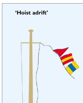
Gadget hauled up on another halyard to try to recover a hoist that has been let go
